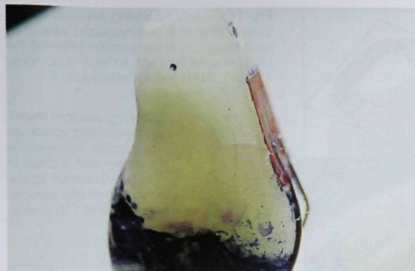
Fig 9 Photomicrograph of a veneered (VEN) specimen (original magnification \times 3 ) after the dye infiltration test. Due to simulated aging, a crack developed within the ceramic and propagated into the junction between the ceramic and the Class III restoration.
